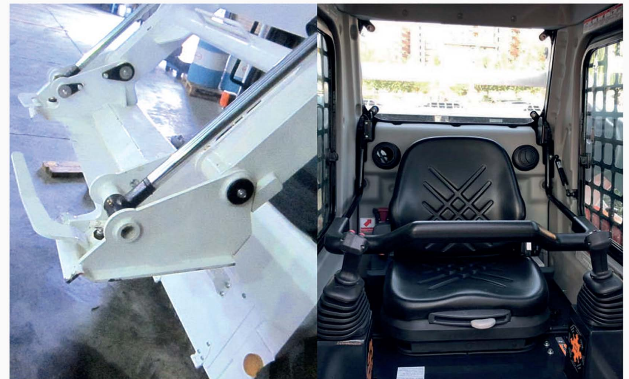
simple attachment system lets you switch from a bucket to a sweeper or to a dozer .blade in seconds
